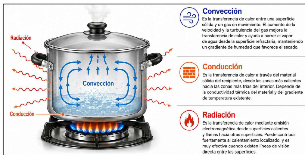
Figure 3. Heat transfer mechanisms during drying. Conduction, convection, and radiation act simultaneously, although convective circulation is essential for distributing heat and removing moisture.
